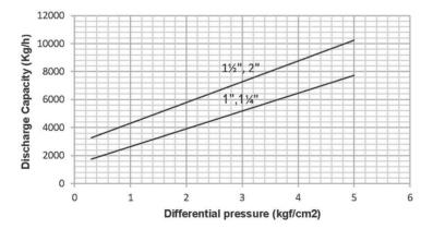
Note: Capacities shown are based on discharge at saturation temperature. In 442FT when discharging sub-cooled condensate, the air vent provides extra capacity. Under start up conditions the thermostatic air vent will be open, and will provide additional condensate capacity to outlet.
